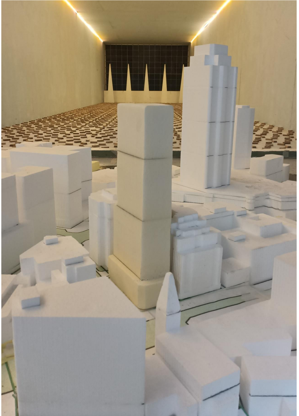
Figure 1i: Photograph of the Wind Tunnel Model (Alternative Envelope A, view from the south-east)
