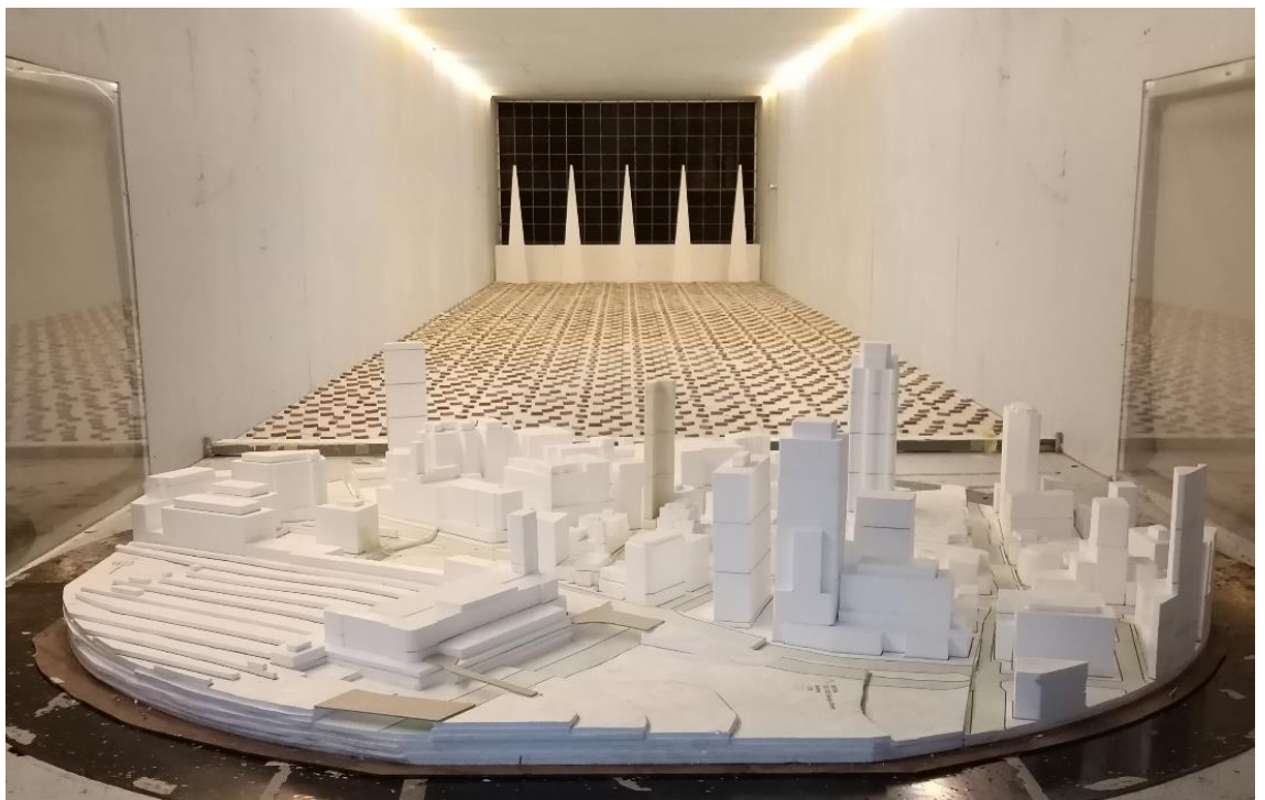
Figure 1b: Photograph of the Wind Tunnel Model (Proposed DCP Envelope, view from the east)
